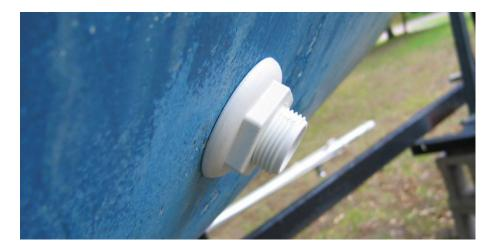
I tried to thread a valve onto here but there weren't enough threads to even hand tighten it. I figure that the combined thickness of the hull and mounted backing plate would have to be about one inch to be able to mount the valve. The picture below is showing a few more threads than the photo above. To expose more threads I would have to remove more material from the inside of the hull.
